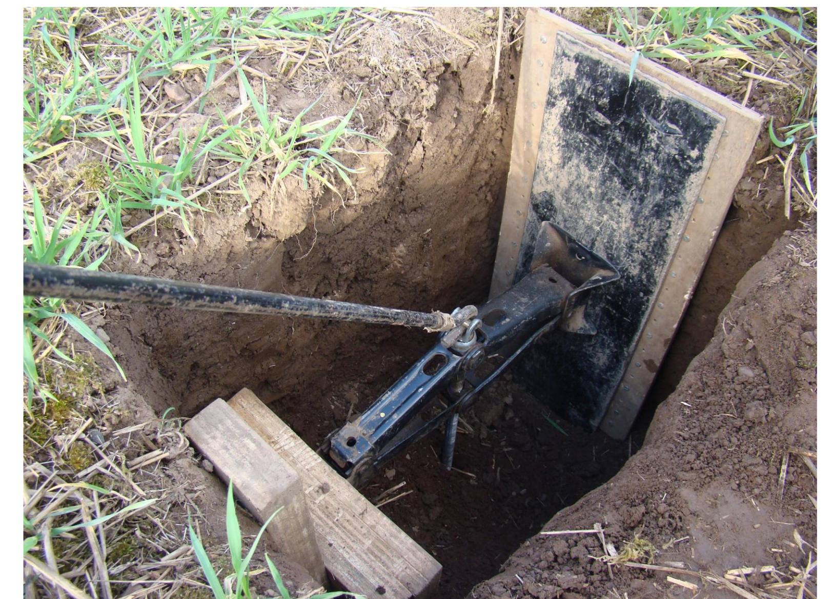
Profiles are collected with the aid of a scissor-jack
