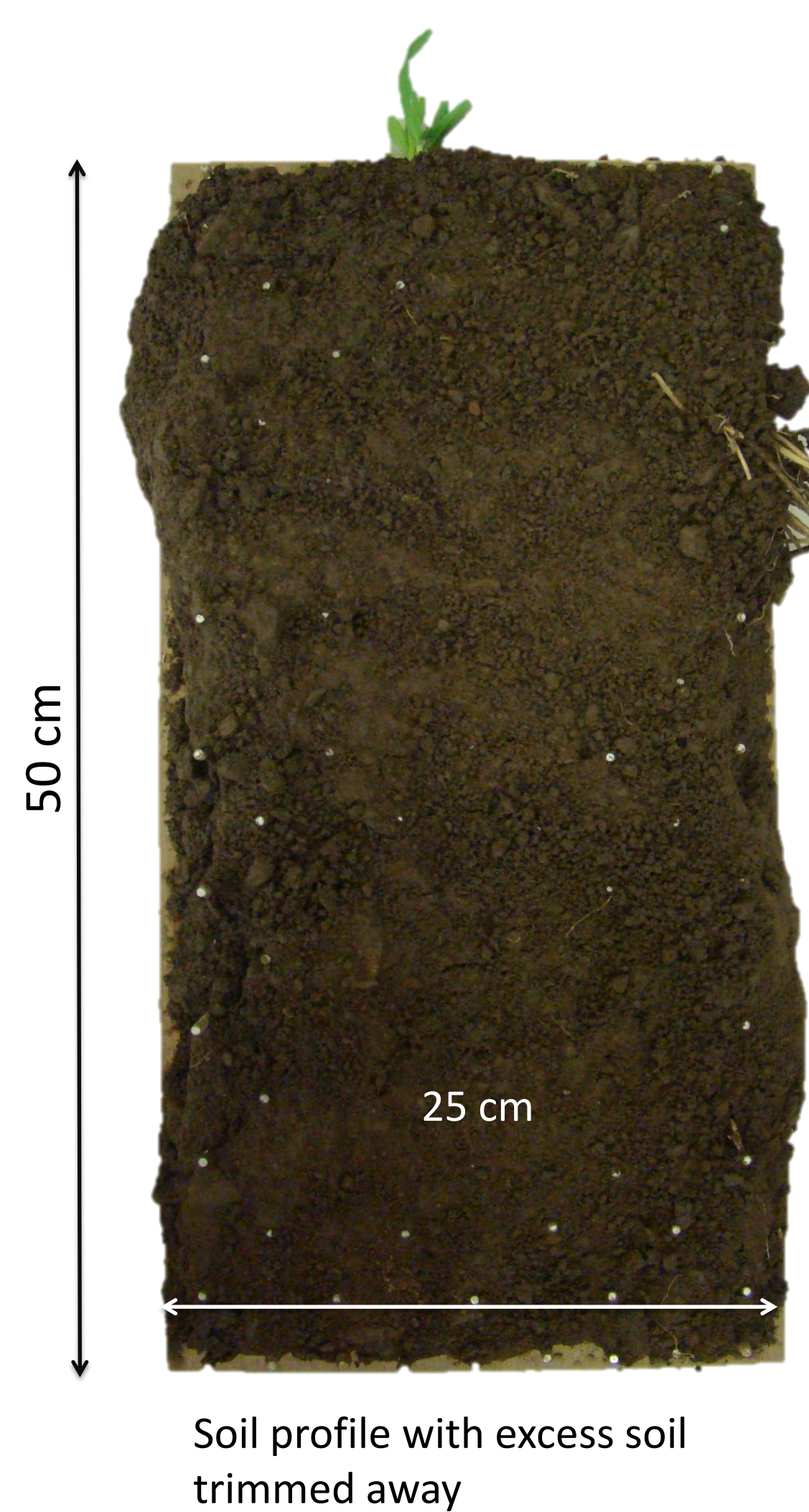
Profiles are collected with the aid of a scissor-jack
